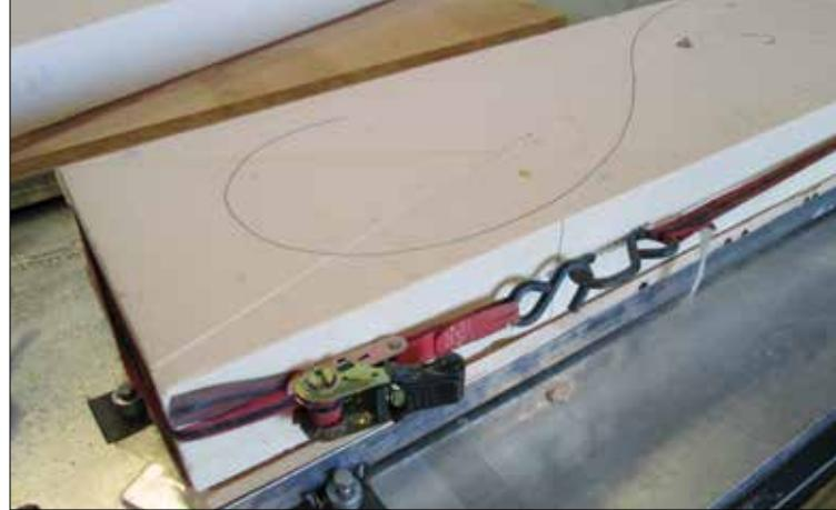
(L) Mold frame for the horizontal stabilizer with CNC-bed locator tabs. Construction adhesive has just been applied for application of the particle board base. (R) Frame bolted to CNC. Due to the high cost of tooling foam, the cutoffs from the wing molds were reassembled into a rectangle for the horizontal stabilizer mold. A ratchet strap holds the foam tight while the epoxy bonding it to the base board cures.
