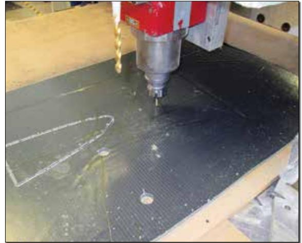
Ribs are CNC'd from a panel of carbon-Divinycell-carbon sandwich. The panel is lightly bonded with contact cement to a sacrificial bed of MDF, which is itself temporarily clamped to the CNC table during the operation. After machining, parts are easily removed from the MDF with a drywall spatula. For small parts like this, a small .125-inch toolhead is used.
