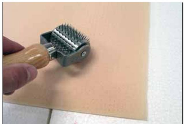
The last component to be CNC'd is the wing core. As with the carbon sandwich panel, quarter-inch Divinycell is lightly bonded with 3M Super 77 to the sacrificial MDF bed. Once the edges are cut and beveled, the Divinycell is carefully pried loose with a drywall spatula. The wing cores are then rolled with a porcupine roller to ensure a good bond to the carbon skin.
