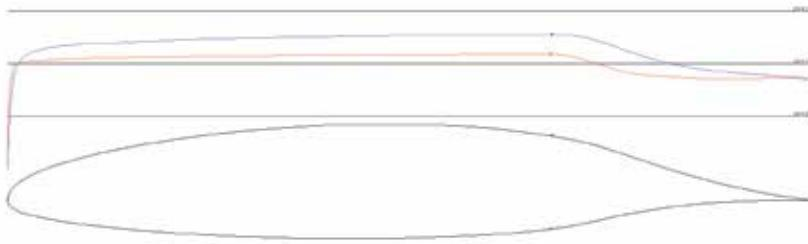
Figure 2. Unmodified NLF 0414 profile with velocity distribution, plotted with AeroFoil V3.2. (Courtesy Donald Reid—[aerofoilengineering.com](http://aerofoilengineering.com))
