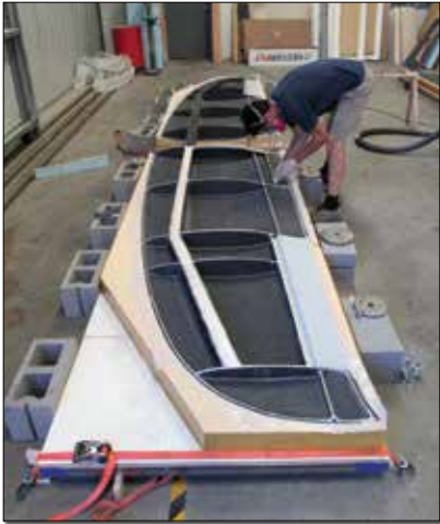
(L) Structural adhesive is applied to the lower (here facing upwards) surface bond lines (spar, ribs, trailing edge and leading edge flashing) and the right lower skin is dropped in place. (R) The leading edge is Clecoed (Cleco holes were drilled earlier during initial fitting) and weights are applied to the trailing edge. Here Paulo inspects the root rib bond line.
