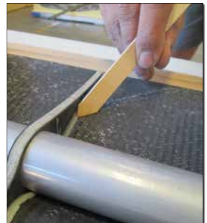
Elsewhere (ribs, trailing edge, etc.) structural adhesive is applied pastry-bag style (L) and filleted with a tongue depressor (R). These pics show construction of the aileron, in which the aluminum torque tube also doubles as the aileron spar. (Only the tip of the pastry bag is visible in the photo on the left, but it's simply a heavy duty freezer bag filled with adhesive and a small tip of the corner cut out. This allows the adhesive to be squeezed out in a clean, controlled fashion.)
