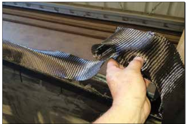
Three layers of bias carbon tape are applied to the leading edge. Bias requires careful handling as it has a tendency to deform easily, although this is the same property that makes it great for taping high-curvature areas like the leading edge.
