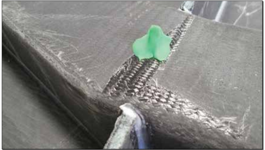
(L) Ribs and spar have been bonded to the top wingskin and are held with "gravity clamps" while the resin cures. (R) Finally, the bottom skin is prepared for bonding. Play-Doh pyramids are located along the spar to plumb the gap between spar and skin, and determine the quantity of structural adhesive necessary to fill the gap. When the bottom skin is temporarily fitted in place, it smashes the Play-Doh down, thus providing an indication of the skin-spar gap.
