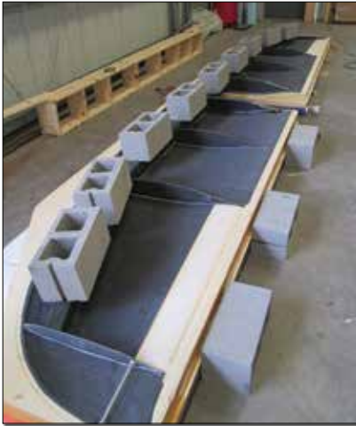
(L) Ribs and spar have been bonded to the top wingskin and are held with "gravity clamps" while the resin cures. (R) Finally, the bottom skin is prepared for bonding. Play-Doh pyramids are located along the spar to plumb the gap between spar and skin, and determine the quantity of structural adhesive necessary to fill the gap. When the bottom skin is temporarily fitted in place, it smashes the Play-Doh down, thus providing an indication of the skin-spar gap.
