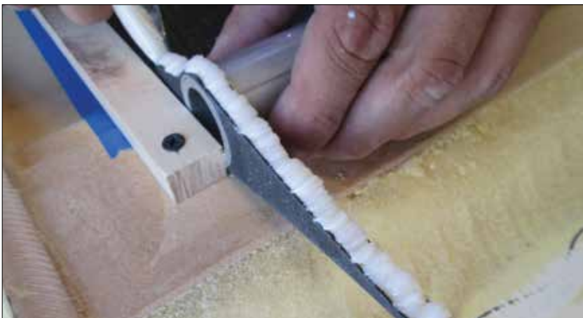
Elsewhere (ribs, trailing edge, etc.) structural adhesive is applied pastry-bag style (L) and filleted with a tongue depressor (R). These pics show construction of the aileron, in which the aluminum torque tube also doubles as the aileron spar. (Only the tip of the pastry bag is visible in the photo on the left, but it's simply a heavy duty freezer bag filled with adhesive and a small tip of the corner cut out. This allows the adhesive to be squeezed out in a clean, controlled fashion.)
