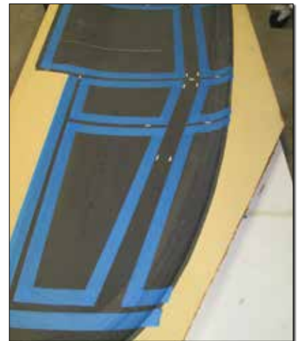
(L) Tacky tape is used to locate the bond line of the spar and ribs by placing strips of tacky tape paper-side down on the spar (wax paper has been removed from the upper surface) and then again temporarily fitting the skin in place. (R) When the skin is removed, the tacky tape sticks to the skin and shows the location of spar and ribs for bond line taping.
