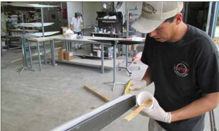
(L) The foam core of the ribs is troughed with a core resector for bonding. This is done immediately before bonding, since the foam has a tendency to spring back after a few days. Once all peel ply has been removed, the ribs and spar are ready to be bonded to the skins. (R) The resector is simply made from hardware store aluminum channel and 1-inch washers.
