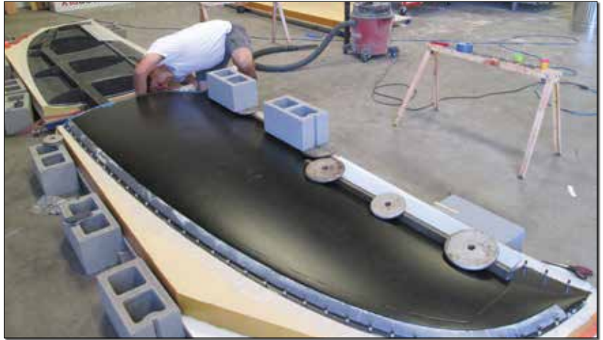
(L) Structural adhesive is applied to the lower (here facing upwards) surface bond lines (spar, ribs, trailing edge and leading edge flashing) and the right lower skin is dropped in place. (R) The leading edge is Clecoed (Cleco holes were drilled earlier during initial fitting) and weights are applied to the trailing edge. Here Paulo inspects the root rib bond line.
