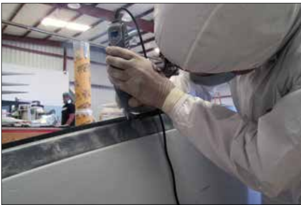
After the bottom skin bonds cure, the wing is placed leading edge up on a stand and the leading edge flashing is removed with a diamond disc Dremel. This creates lots of carbon fiber dust, so a full safety suit and respirator are essential. The leading edge peel ply is also removed at this point, and following a bit of sanding, the leading edge is ready to be taped.
