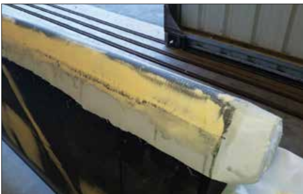
After the final layer of tape, a layer of epoxy and microballoons is applied to smooth the transition between the tape and the wing mold joggle, followed by peel ply. After cure, the wing is block sanded smooth. This removes any irregularities in the leading-edge region, as well as the primer orange peel.
