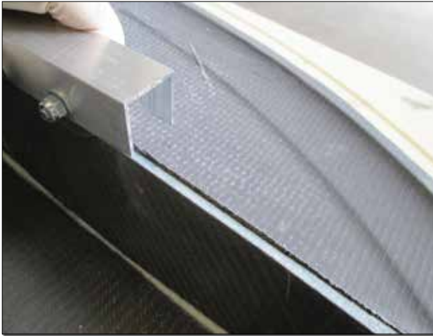
(L) The foam core of the ribs is troughed with a core resector for bonding. This is done immediately before bonding, since the foam has a tendency to spring back after a few days. Once all peel ply has been removed, the ribs and spar are ready to be bonded to the skins. (R) The resector is simply made from hardware store aluminum channel and 1-inch washers.
