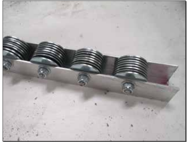
(L) The foam core of the ribs is troughed with a core resector for bonding. This is done immediately before bonding, since the foam has a tendency to spring back after a few days. Once all peel ply has been removed, the ribs and spar are ready to be bonded to the skins. (R) The resector is simply made from hardware store aluminum channel and 1-inch washers.
