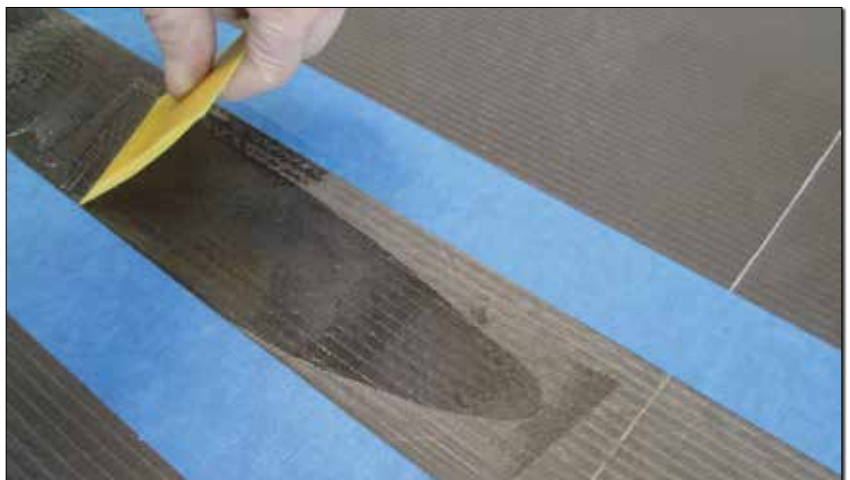
(L) All bond lines are taped, scuffed, and wiped with acetone for bonding (including the aluminum aileron spar/torque tube). (R) Just before closeout bonding, the bond lines are painted with straight epoxy to ensure a consolidated skin bond with the structural adhesive.
