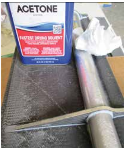
(L) All bond lines are taped, scuffed, and wiped with acetone for bonding (including the aluminum aileron spar/torque tube). (R) Just before closeout bonding, the bond lines are painted with straight epoxy to ensure a consolidated skin bond with the structural adhesive.
